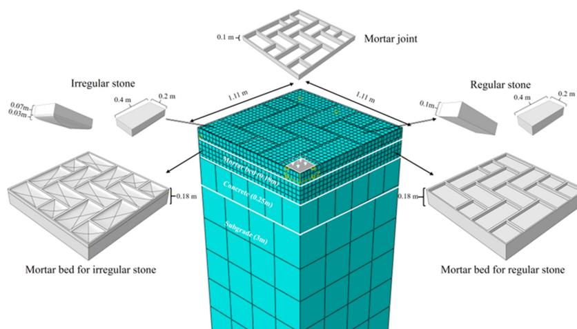
**Figure 7.** Physical model sizes and FEM mesh.
