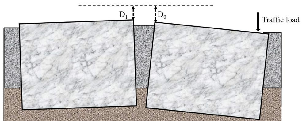
Figure 15. Joint efficiency characterized by the LTE.
