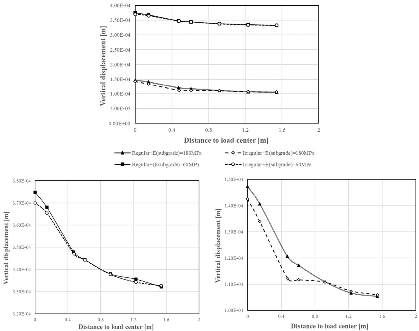
Figure 8. Vertical displacement for the R-SPS and H-SPS.
