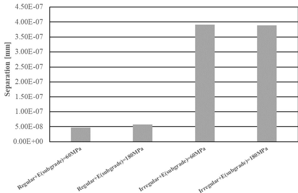
Figure 14. The separation between stone and mortar joints.
