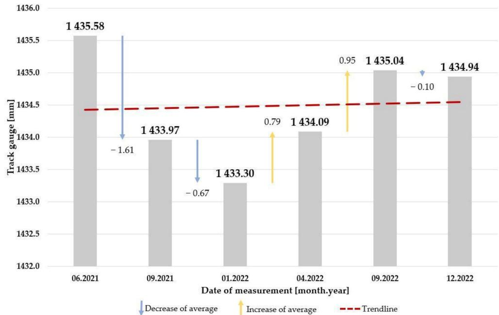
Figure 16. The change of average values of the track gauge in Section #4.
