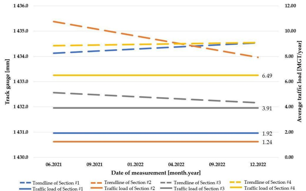
Figure 24. The relationship between track gauge and traffic load in ballasted track systems.
