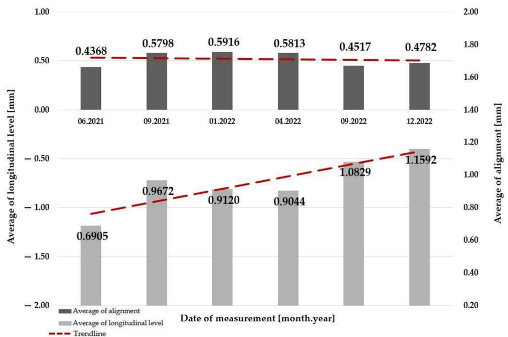
Figure 23. The change of average values of longitudinal level and alignment in Section #7.
