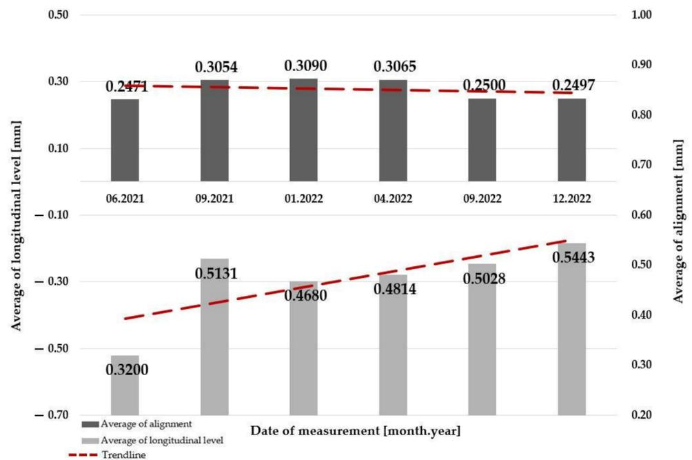
Figure 11. The change of average values of longitudinal level and alignment in Section #1.
