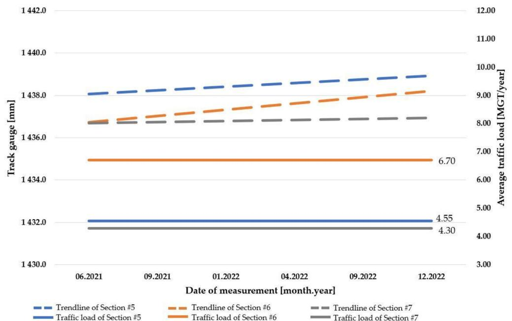
Figure 27. The relationship between track gauge and traffic load in concrete slab track systems.
