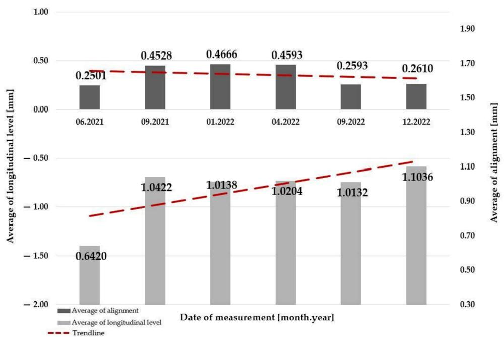
Figure 15. The change of average values of longitudinal level and alignment in Section #3.
