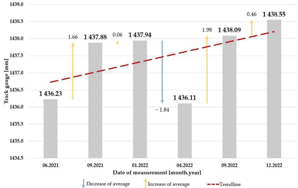
Figure 20. The change of average values of the track gauge in Section #6.
