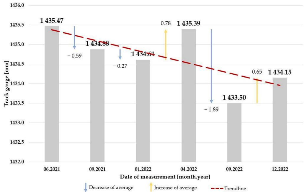
Figure 12. The change of average values of the track gauge in Section #2.
