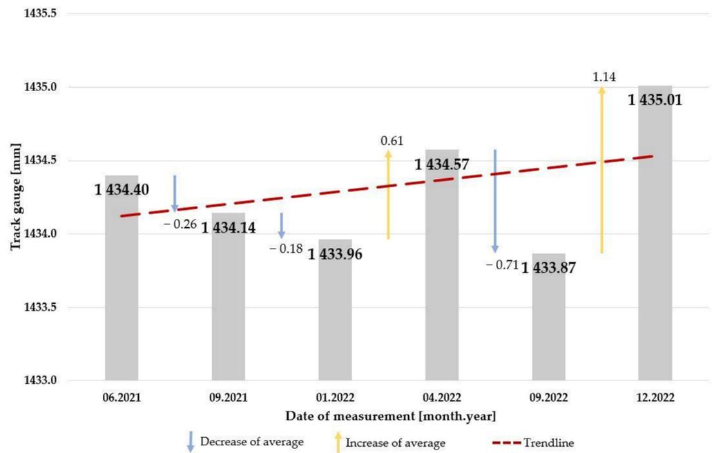
Figure 10. The change of average values of the track gauge in Section #1.
