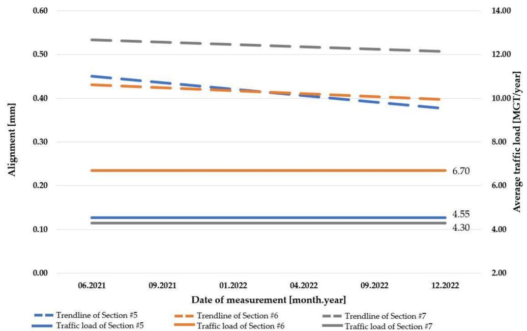
Figure 28. The relationship between alignment and traffic load in concrete slab track systems.
