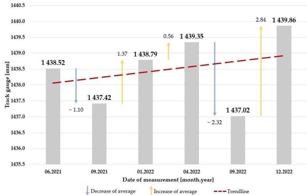
Figure 18. The change of average values of the track gauge in Section #5.
