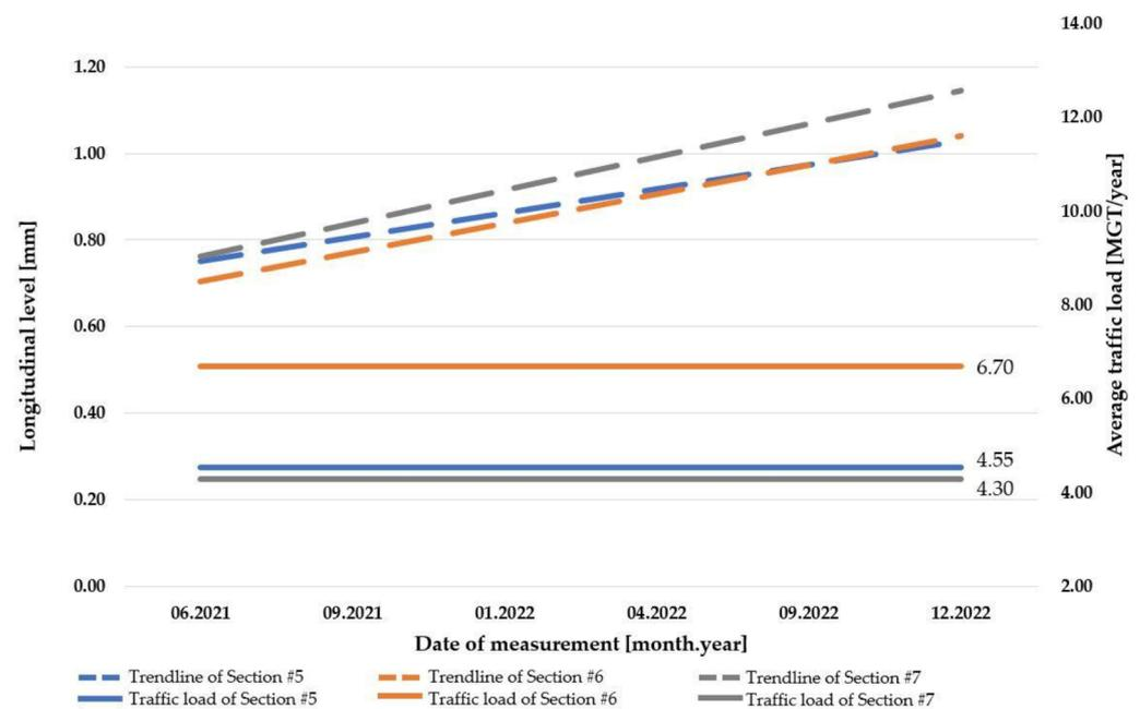
Figure 29. The relationship between longitudinal level and traffic load in concrete slab track systems.
