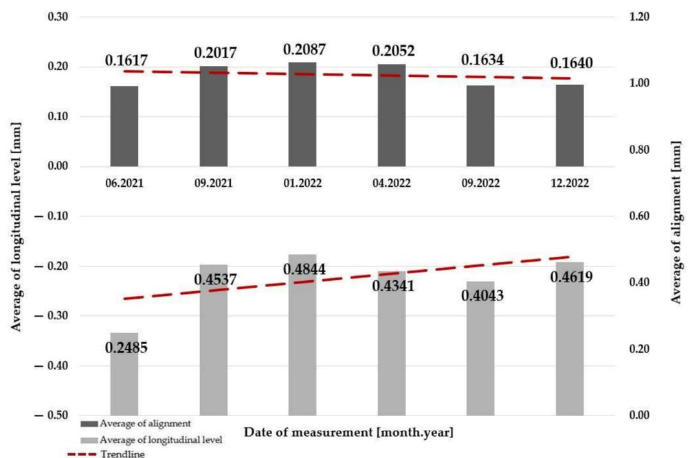
Figure 17. The change of average values of longitudinal level and alignment in Section #4.
