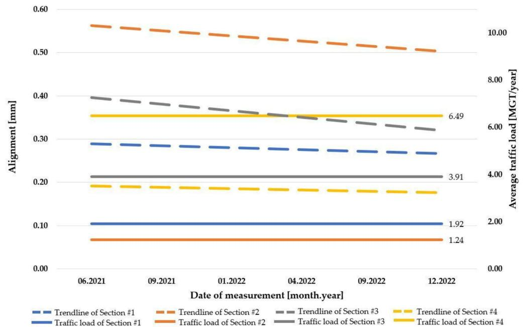
Figure 25. The relationship between alignment and traffic load in ballasted track systems.
