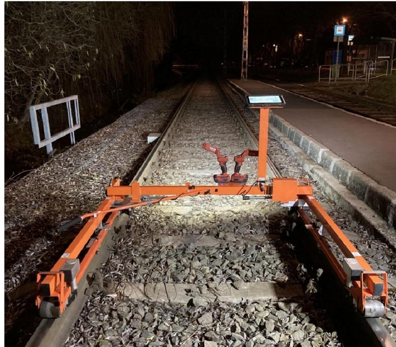
Figure 9. TrackScan 4.01 instrument (own photo).
