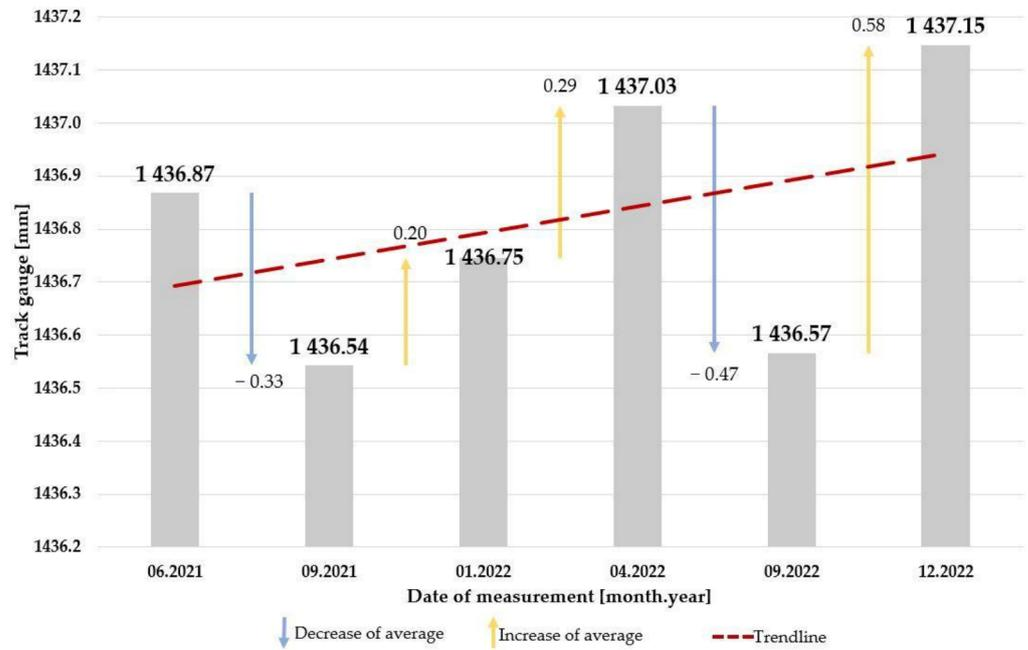
Figure 22. The change of average values of the track gauge in Section #7.
