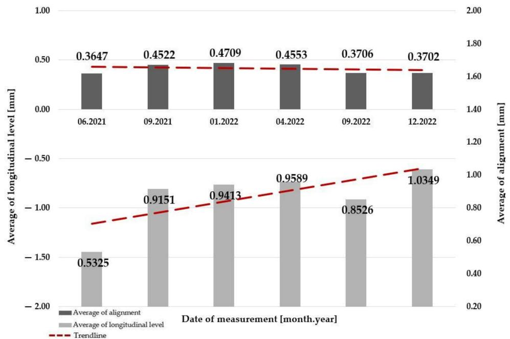
Figure 21. The change of average values of longitudinal level and alignment in Section #6.
