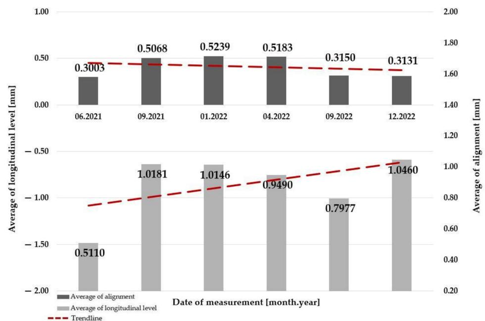
Figure 19. The change of average values of longitudinal level and alignment in Section #5.
