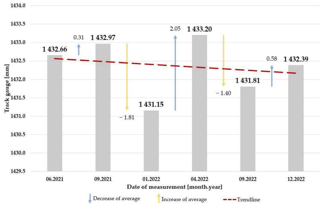
Figure 14. The change of average values of the track gauge in Section #3.
