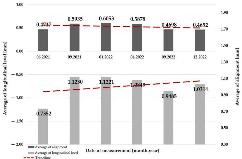
Figure 13. The change of average values of longitudinal level and alignment in Section #2.
