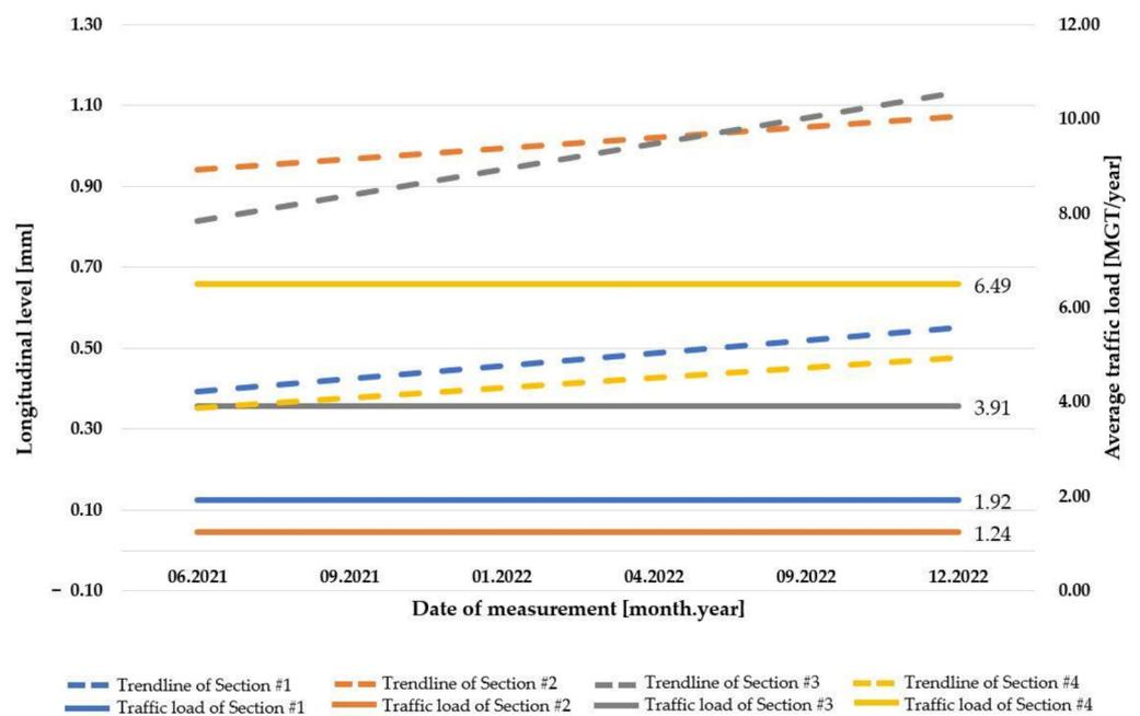
Figure 26. The relationship between longitudinal level and traffic load in ballasted track systems.
