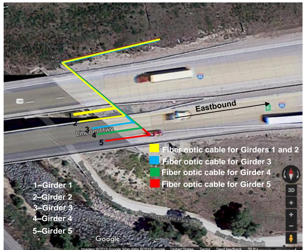
**Figure 9.** Fiber optic system for the bridge with the flange-only array.
