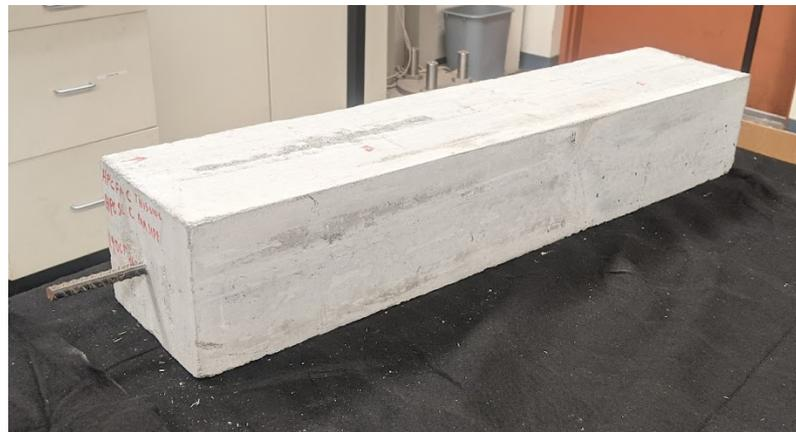
**Figure 1.** Example of a concrete beam sample; note central rebar.
