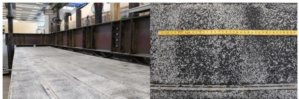
Figure 8. Contrast pattern on slab surface.
