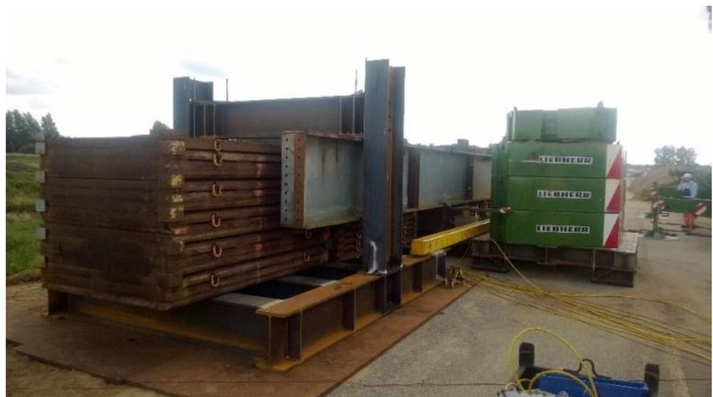
Figure 2. Applied classification loads used for the in situ tests. Standard vehicle A adjacent to standard vehicle B.
