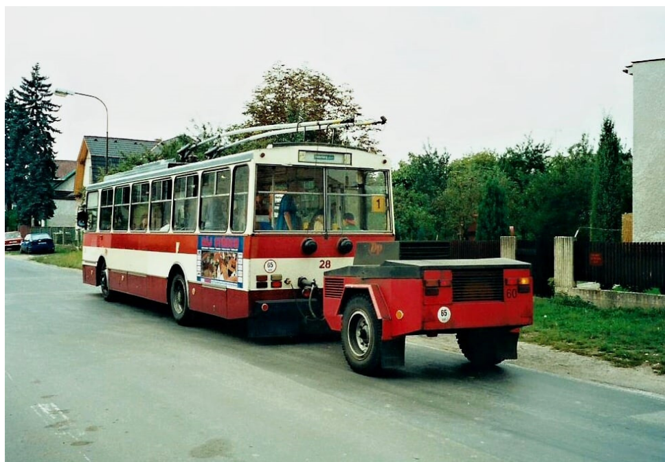
Figure 1. Škoda 14Tr trolleybus with a diesel power generator on the trailer, servicing line no. 1 in Hradec Králové, Czech Republic, from 1994 to 2001 (photo taken by M. Janů).
