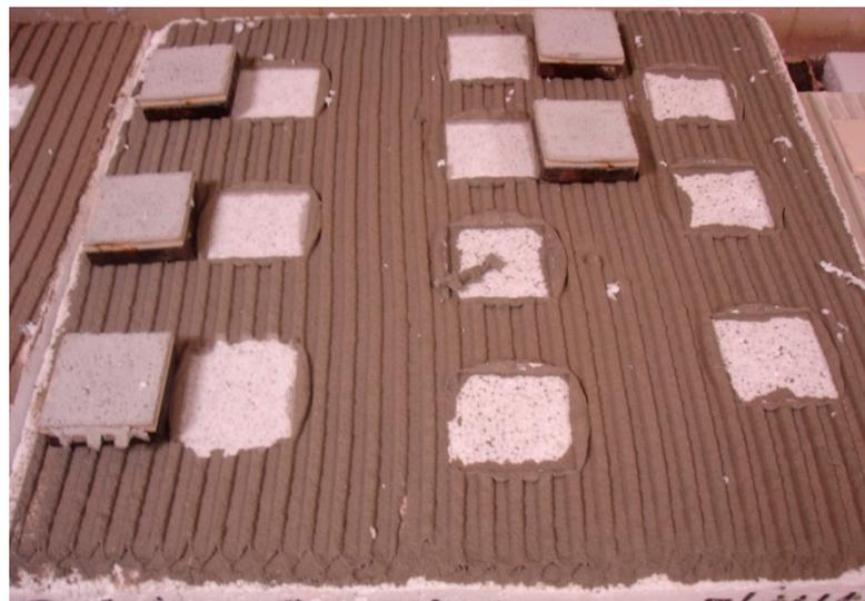
Figure 5. Adhesive strength in EPS (expanded polystyrene) substrate after water immersion (B1).
