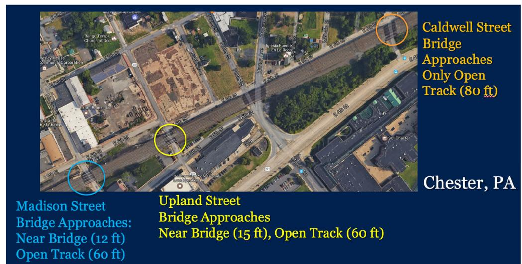
**Figure 1.** Locations of the Three Bridges Selected for Instrumentation in Amtrak's NEC (1 ft = 30.5 cm).
