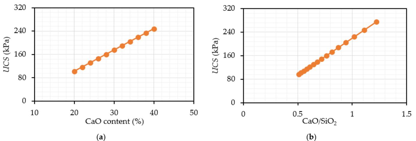
Figure 4. Effect of fly ash characteristics: (a) Effect of CaO content; (b) Effect of CaO/SiO<sub>2</sub>.
