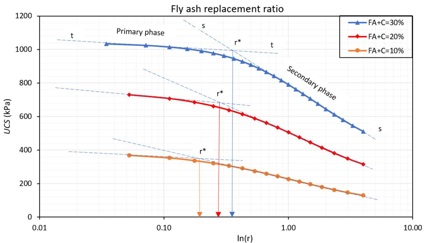
Figure 5. Effect of fly ash replacement ratio.
