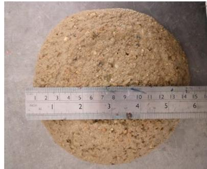
Figure 3. The flow diameter of a CGM with a high amount of GGBS (G91F00M09R00).
