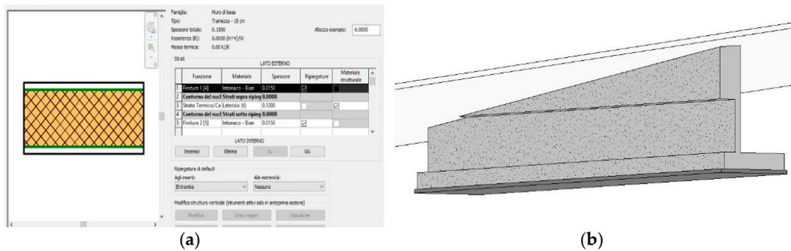
Figure 11. Modeling Retaining walls using Revit: (a) wall family; (b) overlapping wall.
