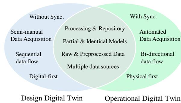
**Figure 7.** Overview of the characteristics of the two archetypes of the Digital Twin structure.
