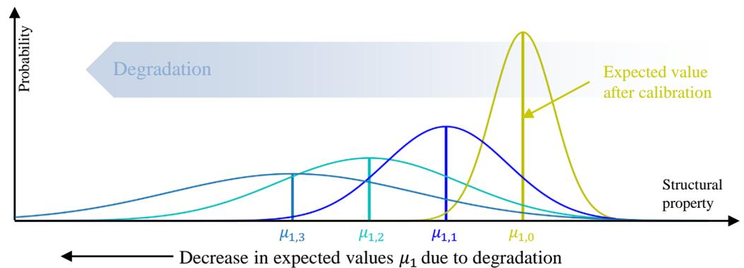
**Figure 4.** Decrease in expected values of structural properties due to in-service degradation overlaid with increasing predictive uncertainty due to fuzzier assumptions regarding experienced load and damage and environmental influences.
