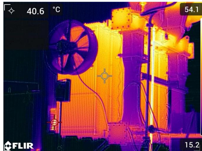
**Figure 8.** Temperature distribution over the radiators and other parts.
