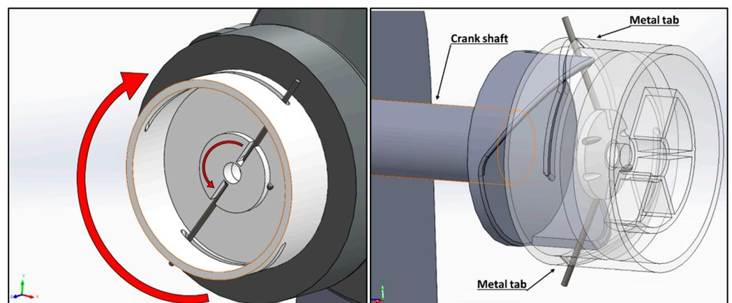
Figure 4. Opposite movement of the shell in relation to the metal tabs during start-up phase (red arrows, left) and metal tabs in lock position (right).
