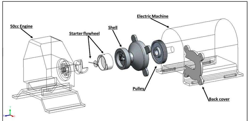
Figure 3. Expanded view of the clutch assembly.
