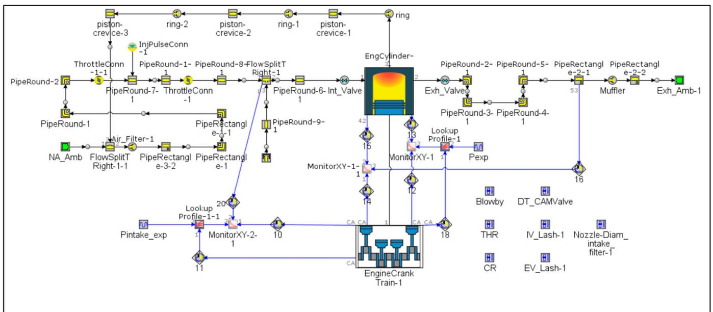
Figure 9. The 0D/1D model of the small-size spark ignition engine.
