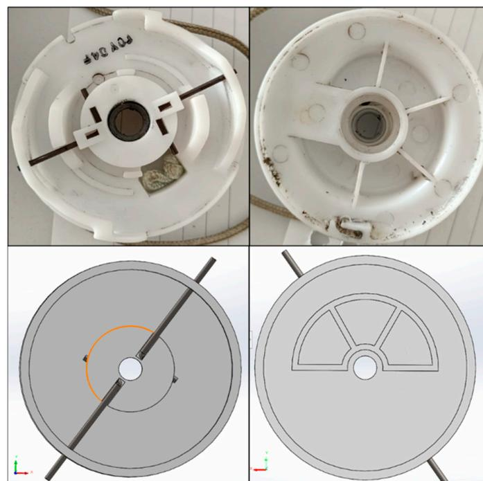
Figure 1. Starter flywheel (top) and CAD model (bottom).
