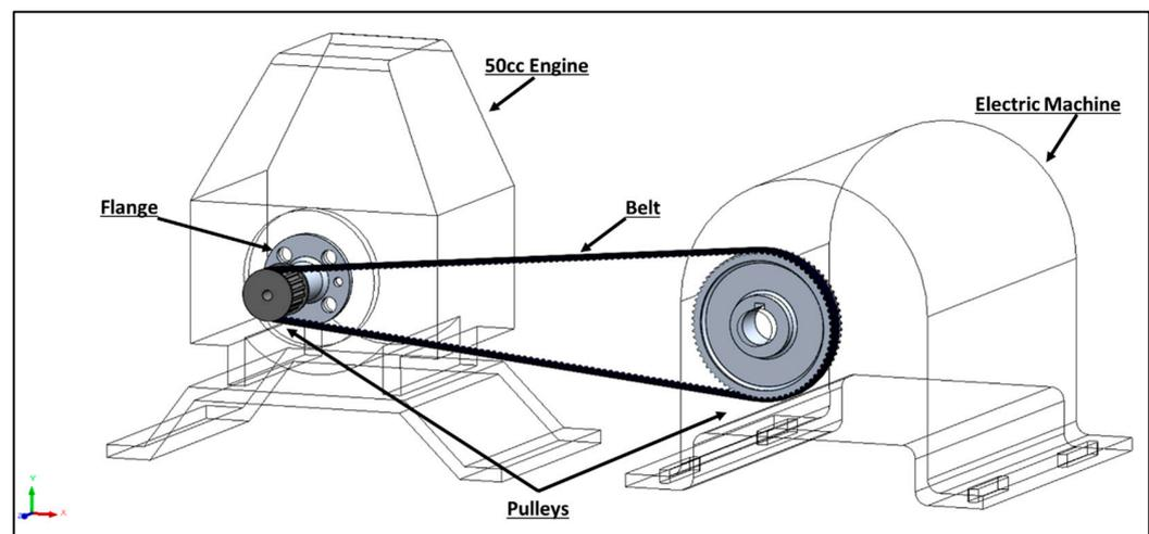
Figure 6. Expanded view of the pulley-belt assembly layout.
