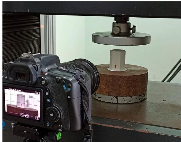
**Figure 2.** A quasi-static set-up for compression test.
