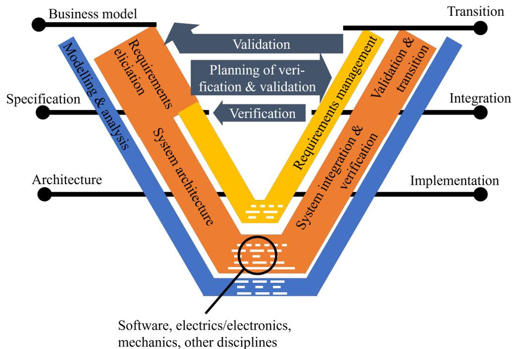
Figure 1. V-Model for development of mechatronic systems according to [4].
