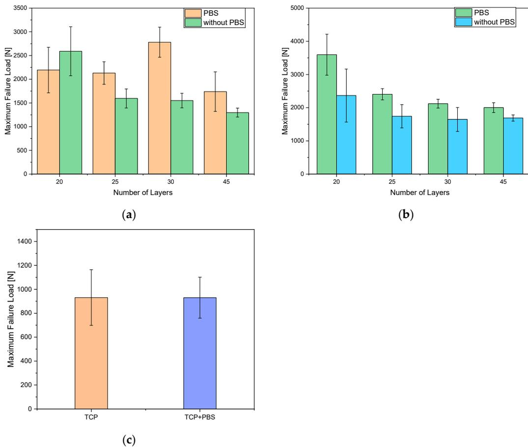
**Figure A3.** Maximum failure load for scaffolds 3D printed with a (a) 0.20 mm needle inner diameter, a (b) 0.25 mm needle inner diameter and (c)  $\beta$ -TCP sinter ceramics scaffolds.
