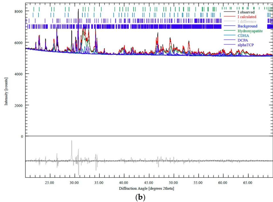
**Figure A2.** Rietveld refinement analysis of the XRD pattern of (a)  $\beta$ -TCP ceramics; (b) CPC (after 3d in water saturated atmosphere); pattern recorded using Bruker D8 Advance with a Cu K $\alpha$  X-ray source.
