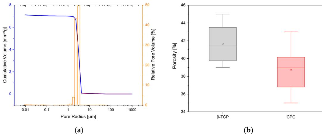
**Figure 5.** (a) Pore size distribution of the  $\beta$ -TCP ceramics determined using Pascal 140 (purple) and 440 (blue curve) mercury porosimeters; (b) boxplot of porosity of  $\beta$ -TCP vs. CPC, with no significant differences.
