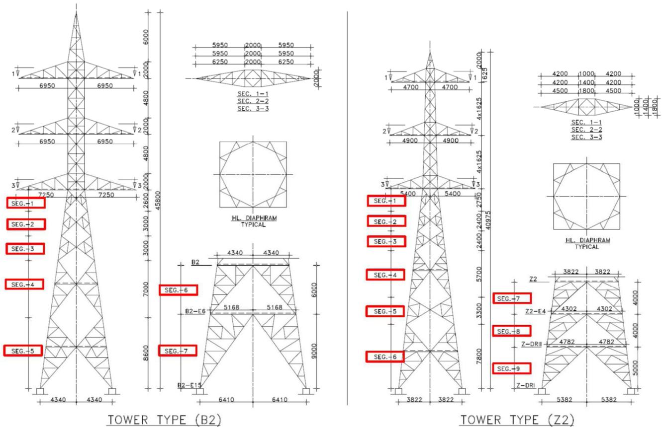
Figure 6. Line diagram of verification tower types: B2 and Z2.
