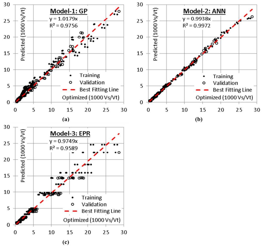
**Figure 5.** Relation between predicted and calculated 1000 Vs/Vt values using the developed models. (a) GP model, (b) ANN-model and (c) EPR model.
