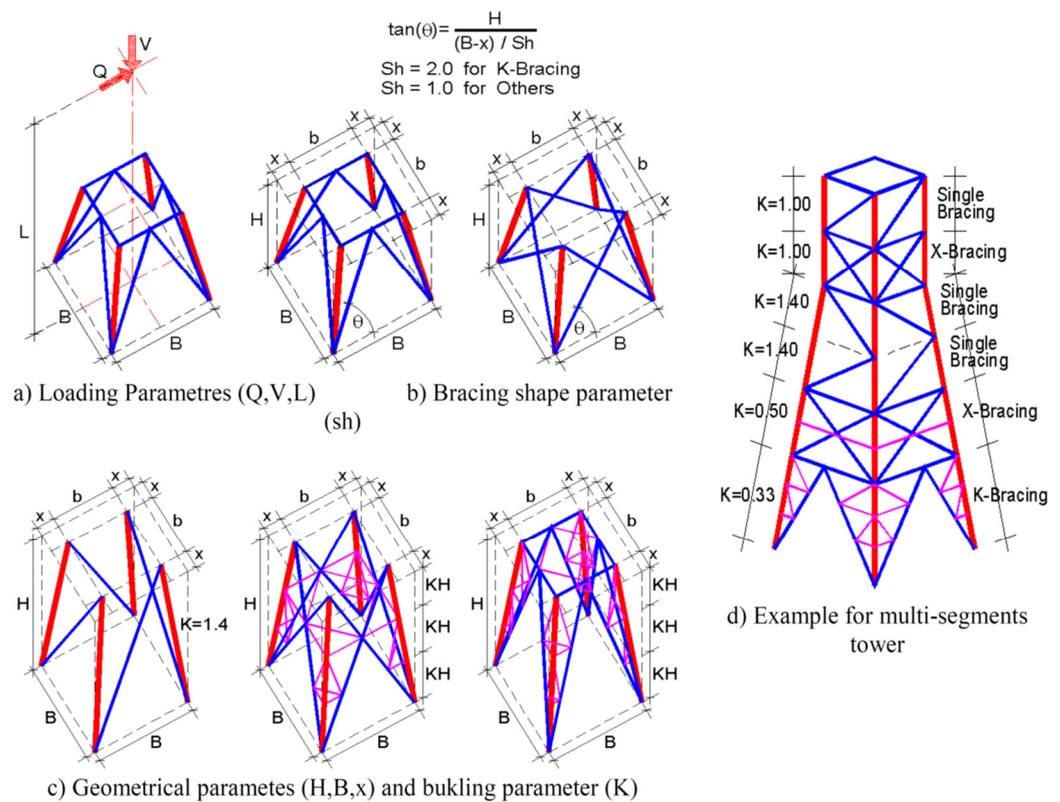
Figure 2. Geometrical and loading parameters.
