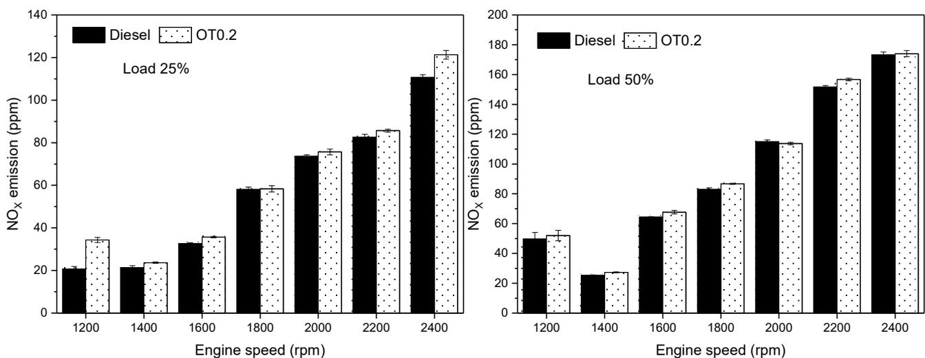
Figure 10. NO<sub>x</sub> emission at various engine speeds.
