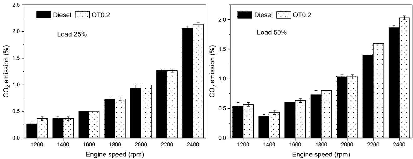
Figure 9. CO<sub>2</sub> emission at various engine speeds.
