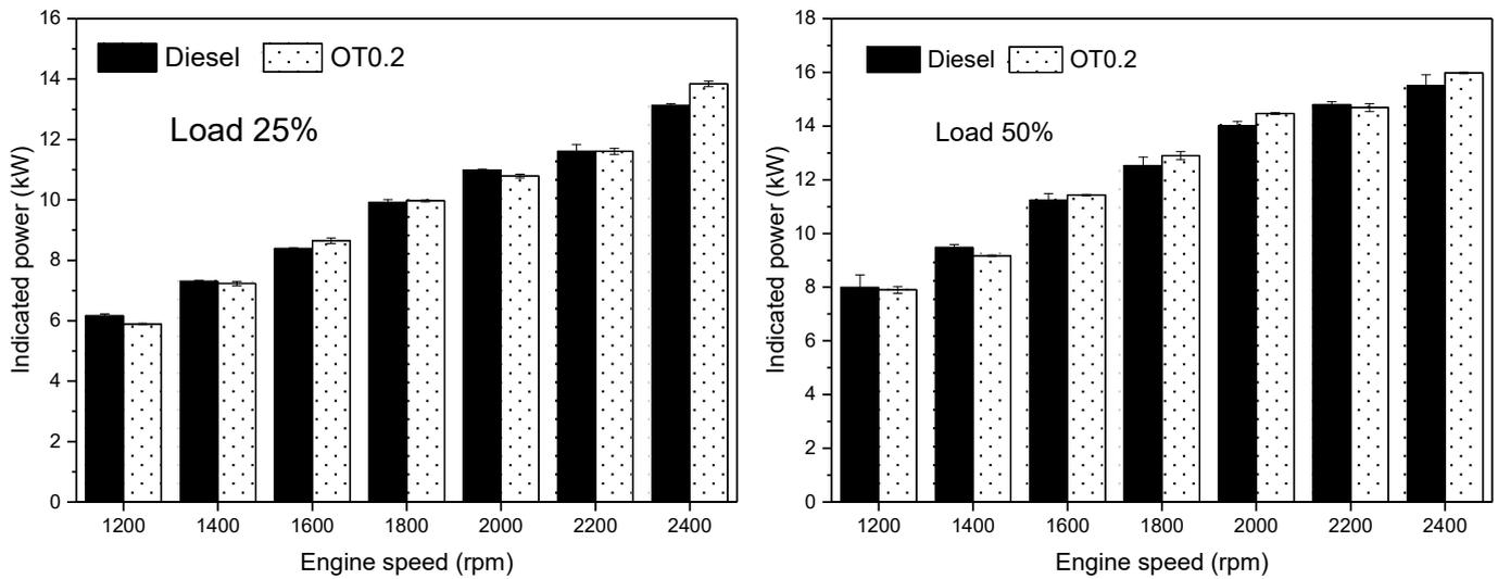
Figure 5. Indicated power at various engine speeds.
