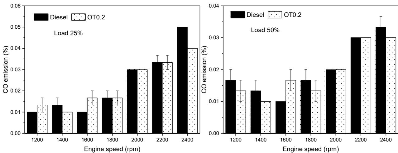
Figure 8. CO emission at various engine speeds.
