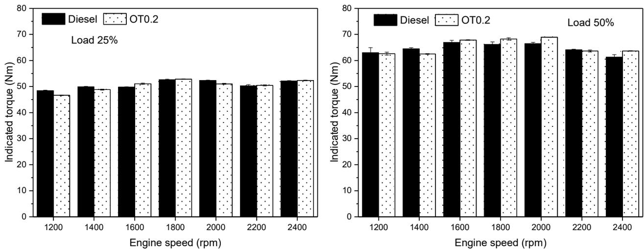
Figure 6. Indicated torque at various engine speeds.
