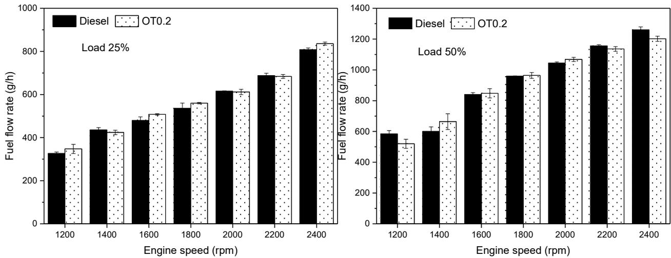
Figure 7. Fuel flow rate at various engine speeds.
