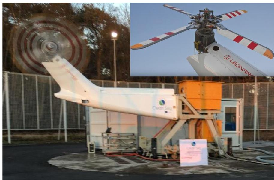
**Figure 9.** Electric Tail Rotor (inset photo showing quadruplex electric drive motor) Undergoing Ground Testing on an Iron Bird Test Rig (Photograph Courtesy of Leonardo).
