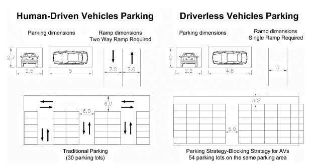
**Figure 9.** Parking Strategy for human-driven vehicles and AVs. (**left**) Conventional parking layout; (**right**) Autonomous Vehicles parking layout (adopted from [68]).
