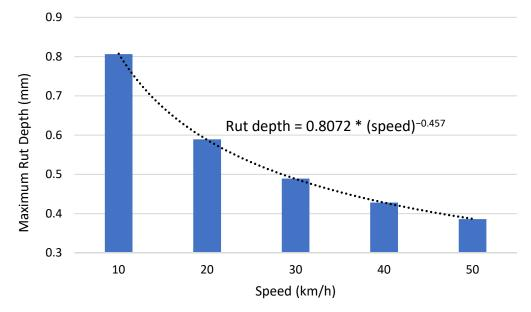
Figure 12. Maximum rut depths with different traffic speed.
