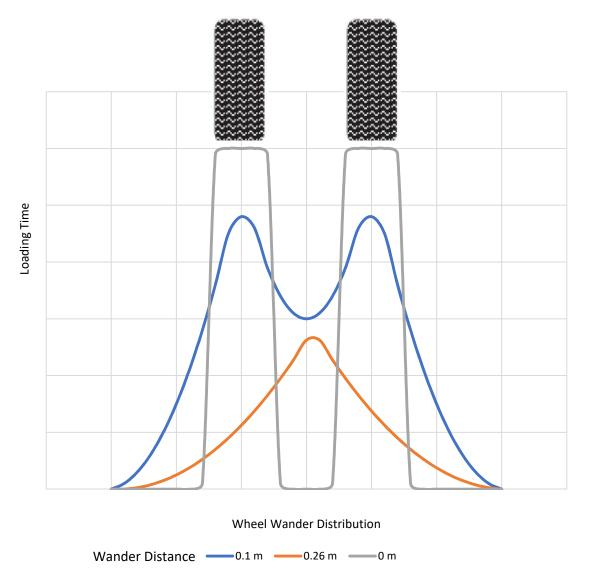
Figure 11. Loading time distributions by the level of wheel wander distance (adopted from [79]).
