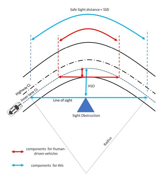
Figure 6. The difference between the components used for Determining Horizontal Sight Distance.
