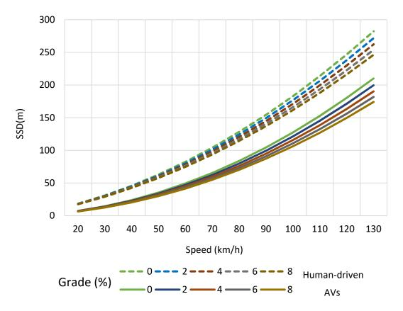
Figure 2. SSD for different upward grades for both human-driven vehicles and AVs.
