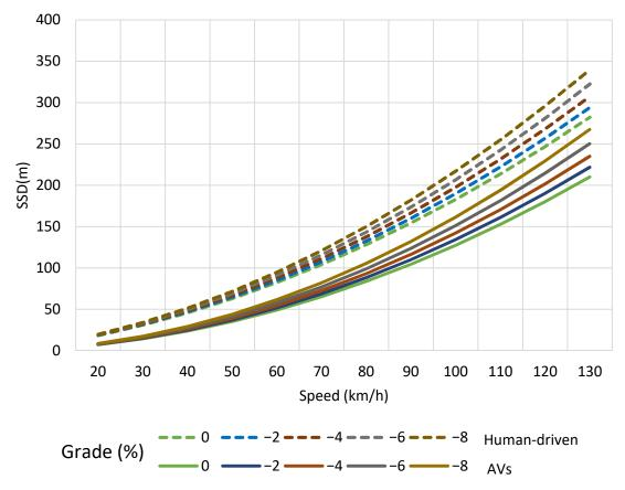
**Figure 3.** SSD for different downgrades for both human-driven vehicles and AVs.
