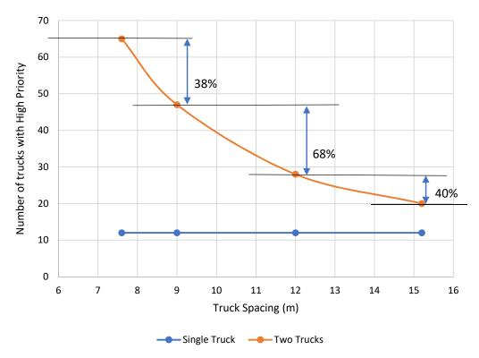
**Figure 15.** Number of high priority bridges for truck type 3S2 at different truck spacing for a single truck and for a platoon of two trucks (adopted from [105]).
