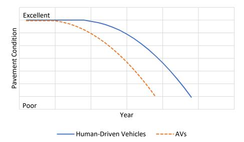
**Figure 13.** Change in pavement conditions over years for human-driven vehicles and AVs with zero wander.
