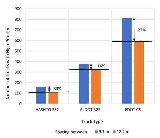
Figure 14. Number of high priority bridges for different truck types and truck spacing (adopted from [103]).
