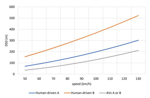
Figure 4. Decision sight distance for the two scenarios A and B for both human-driven and autonomous vehicles.
