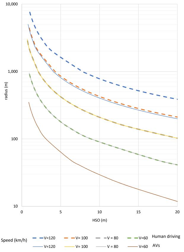
Figure 5. Design Controls for Stopping Sight Distance on Horizontal Curves for human driving and AVs.
