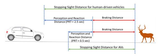
Figure 1. The stopping sight distance for human-driven vehicles and AVs.
