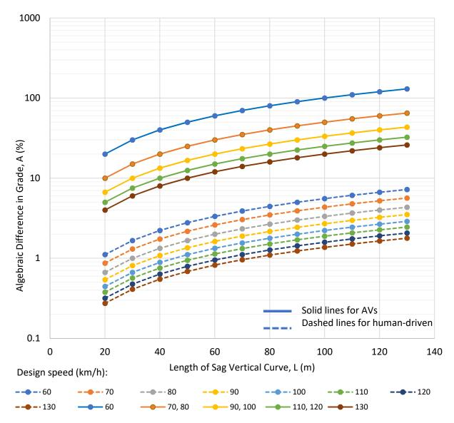
Figure 8. Design Control for Sag Vertical Curves for the case of human-driven vehicles and AVs.
