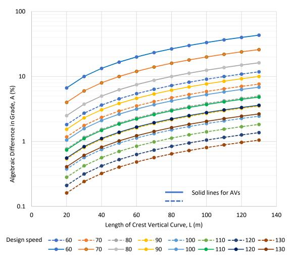
Figure 7. Design Control for Crest Vertical Curves for the case of human-driven vehicles and AVs.
