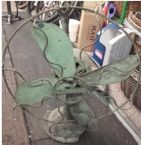
**Figure 2.** An old propeller-type fan (beginning of the 20th century) from an Italian manufacturer of electrical motors: the blades feature no-twist and an elliptical chord distribution. Surprisingly, this table fan appears identical to the sketch presented at the beginning of Wallis' book [8] on fan design.
