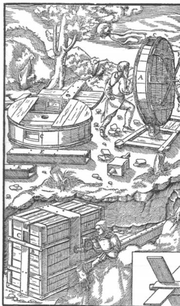
**Figure 1.** The illustration from *De Re Metallica* showing the use of ancient fans for the mechanical ventilation inside an underground mine of the XVI century. Reproduced courtesy of Dover Publications Inc., New York, USA.
