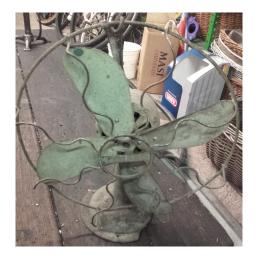
**Figure 2.** An old propeller-type fan (beginning of the 20th century) from an Italian manufacturer of electrical motors: the blades feature no-twist and an elliptical chord distribution. Surprisingly, this table fan appears identical to the sketch presented at the beginning of Wallis' book [8] on fan design.
