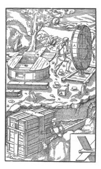
**Figure 1.** The illustration from *De Re Metallica* showing the use of ancient fans for the mechanical ventilation inside an underground mine of the XVI century. Reproduced courtesy of Dover Publications Inc., New York, USA.
