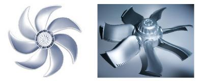
**Figure 8.** Modern low-speed axial fans: notice the innovative features of *Non-radial-stacking-lines*, additional forward sweep and end-plates (on the right rotor) at the tip, and S-shaped trailing edges for noise reduction. Reproduced courtesy of Ziehl-Abegg SE.
