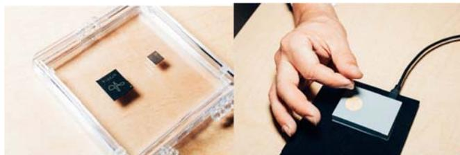
Fig. 8. The challenge of Soli was to shrink radar into the size of a computer chip. PETER MCCOLLOUGH FOR WIRED
