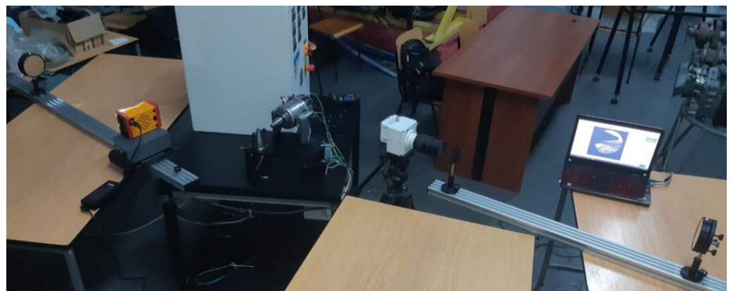
Figure 2. Experimental test bench with aligned Schlieren system.
