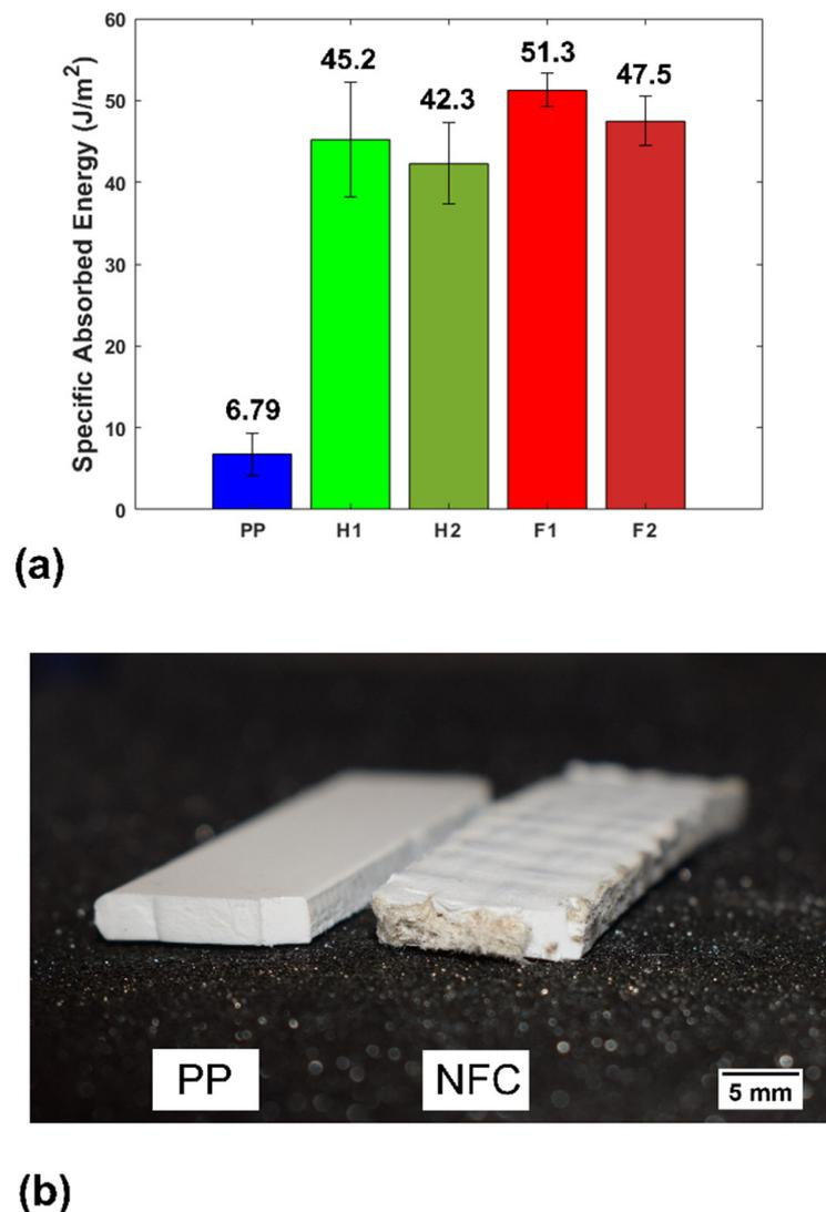
**Figure 6.** (a) Specific adsorbed energy for each sample type and (b) example of sample cross section at the end of the Izod tests.
