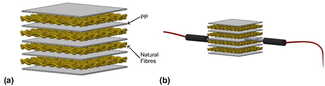
Figure 2. (a) Stacking sequence of composite samples and (b) position of thermocouples.
