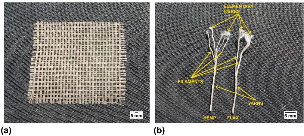
Figure 1. (a) Fabric adopted as reinforcement and (b) magnification of hemp and flax yarn.
