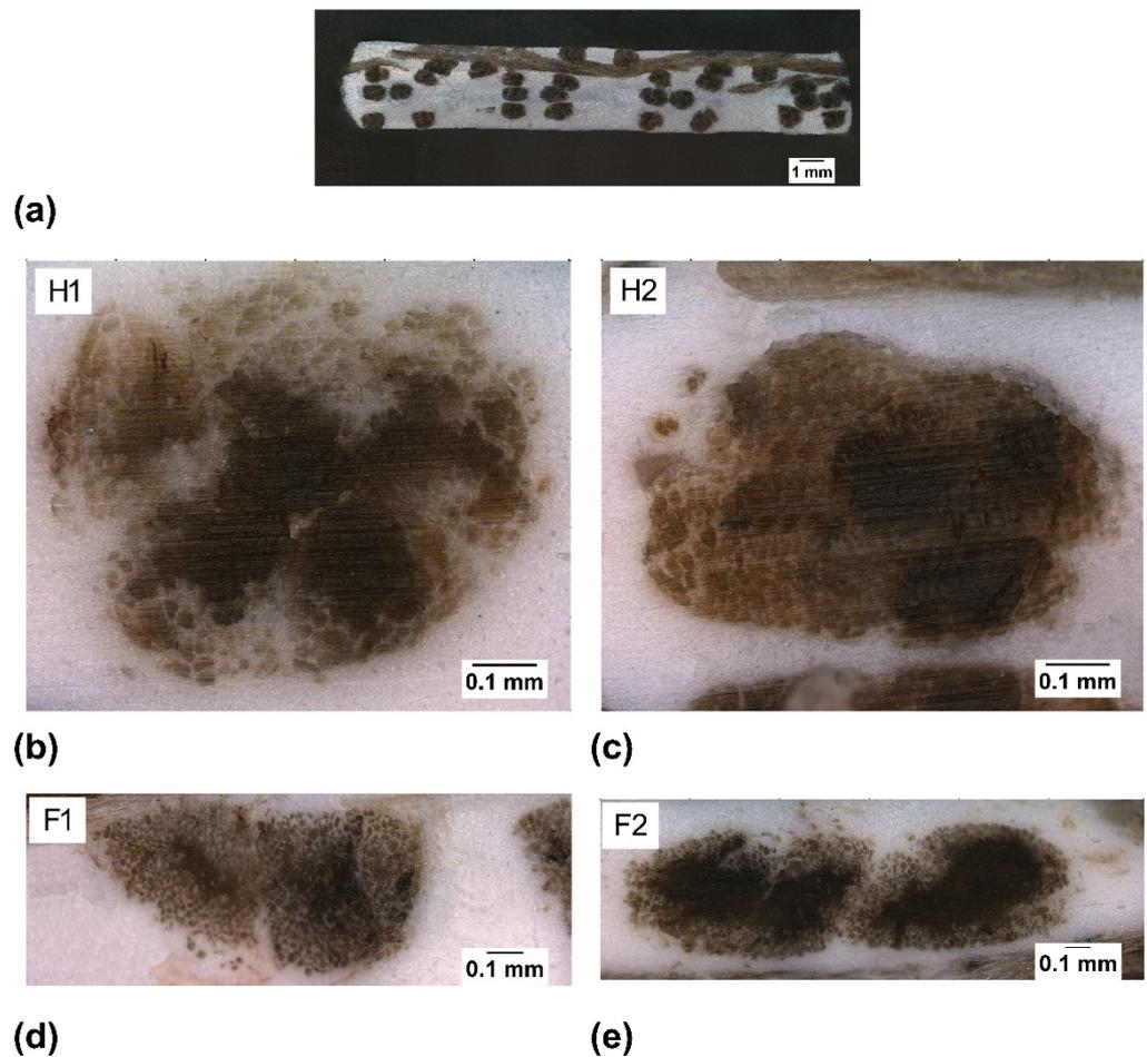
**Figure 4.** (a) Typical cross section of H 1 sample, (b) 10× image magnification of typical yarn of H1, (c) H2, (d) F1 and (e) F2 samples.
