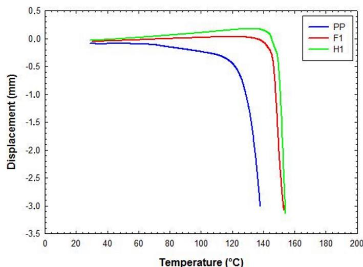
**Figure 10.** Displacement vs temperature curves carried out from HDT tests.
