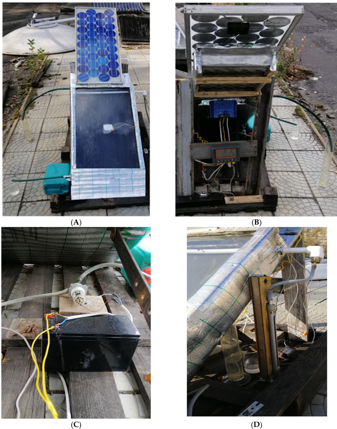
Figure 2. A photograph of the suggested solar still. (A) Front side, (B) back side, (C) micro pump and battery, (D) flow meter.
