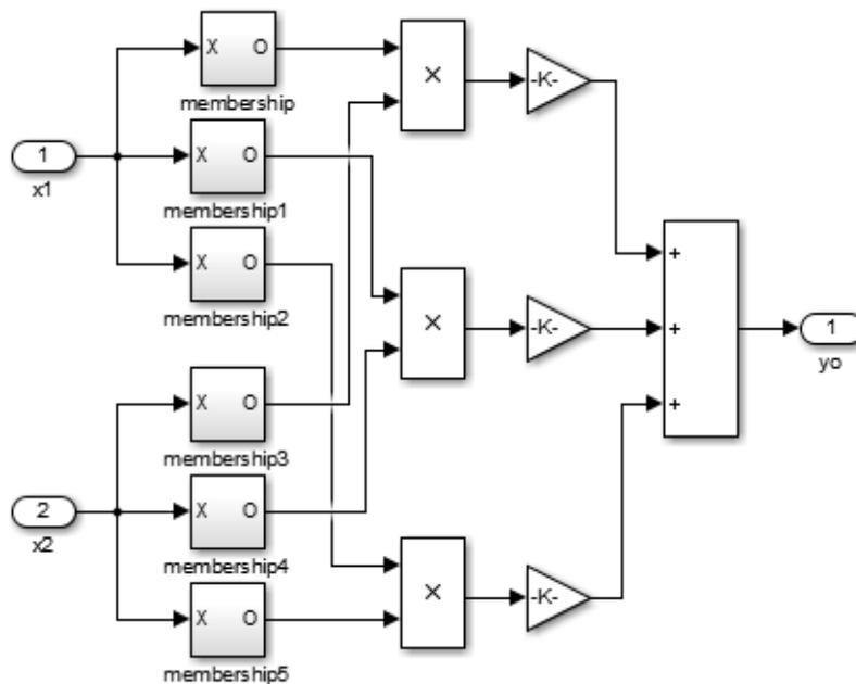
**Figure 7.** Simulink model of the FNN controller.
