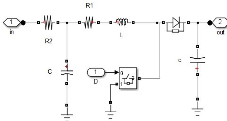
**Figure 6.** Simulink model of the boost converter.
