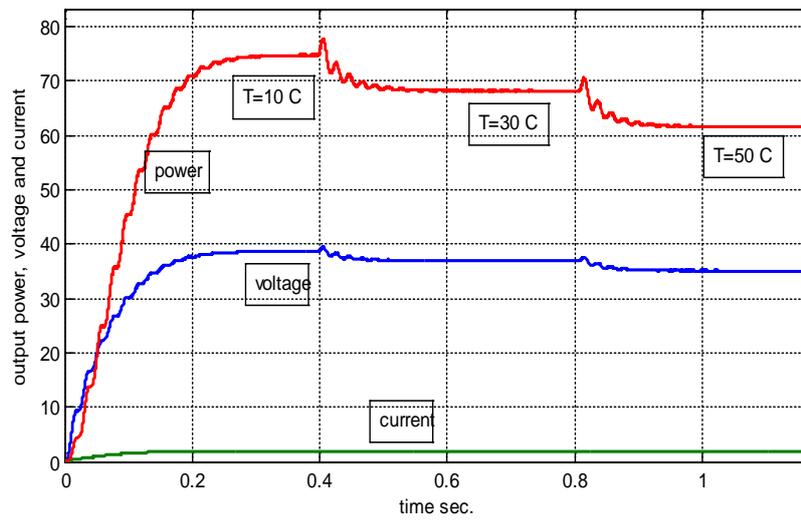
Figure 10. The boost converter output responses at  $G = 500 \text{ W/m}^2$
