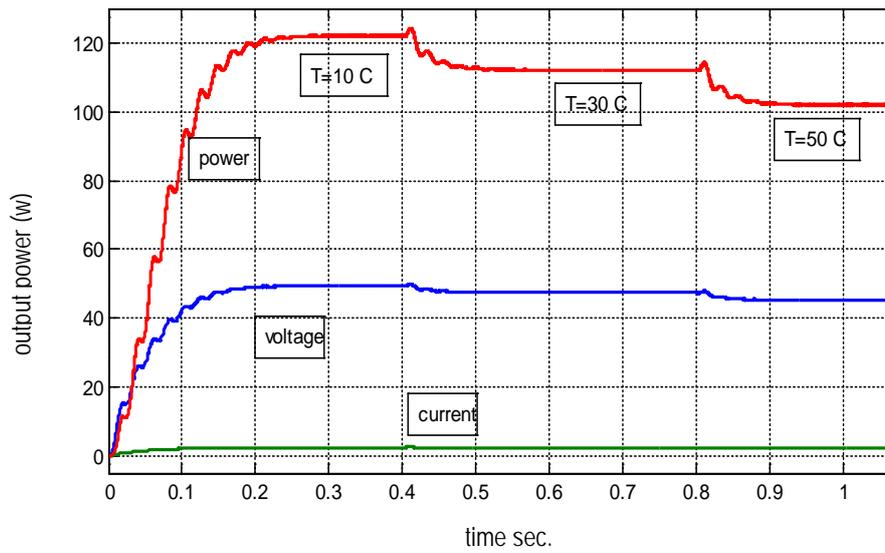
Figure 9. The boost converter output responses at  $G = 800 \text{ W/m}^2$
