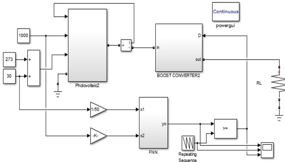
Figure 5. The Simulink model of the overall PV system with the proposed controller based on MPPT.
