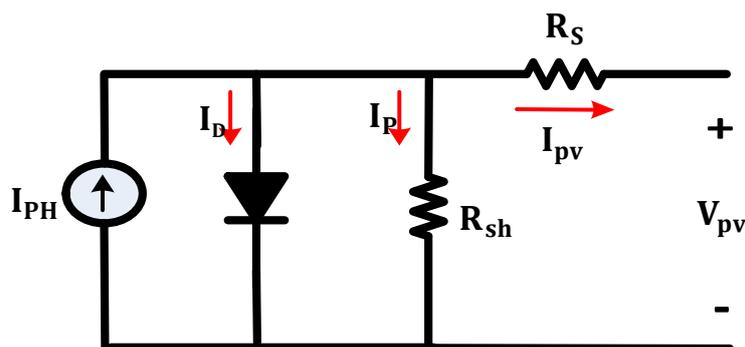
Figure 1. Single-diode model.
