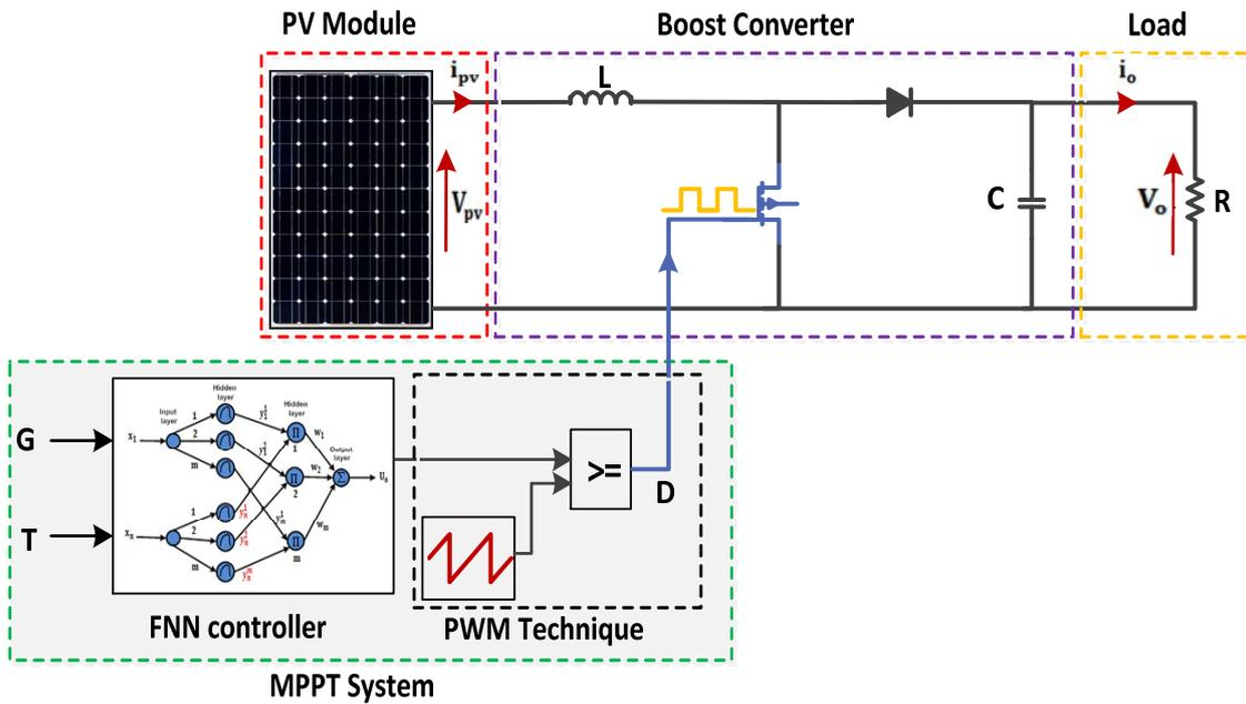
Figure 4. Block diagram of the PV system with an FNN controller based on MPPT.
