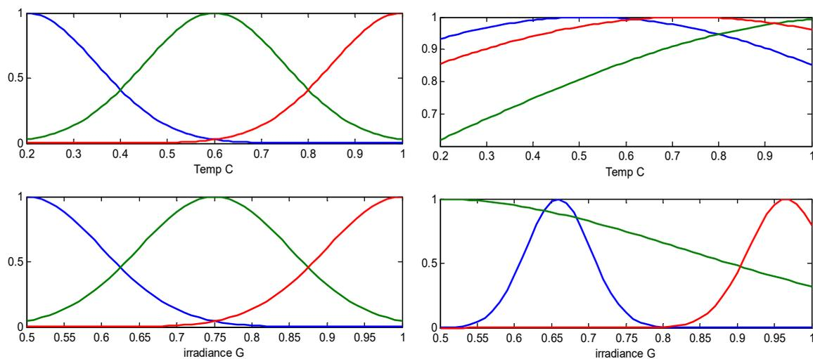
**Figure 8.** Membership functions of the FFN controller before and after training.
