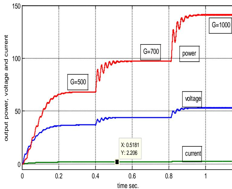
Figure 11. The boost converter output responses at T = 30 °C.
