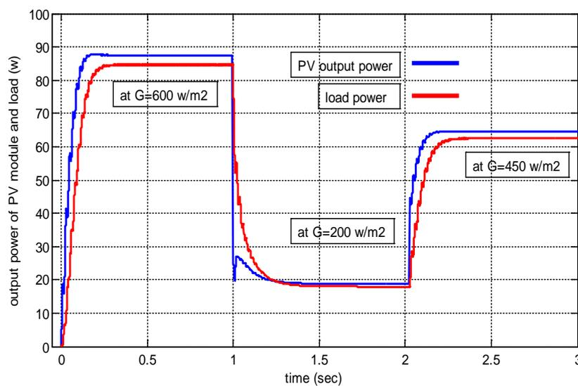
Figure 12. Load power tracking to the PV output power at T = 30 °C.
