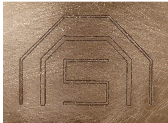
Figure 11. An image of the octagonal shape used to verify feature accuracy.
