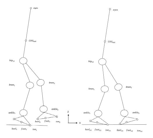
Figure 2. The robot: sagittal plane—single and double stance.
