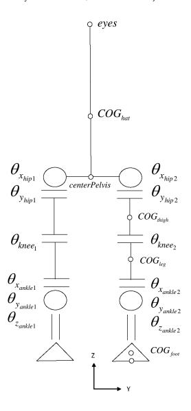
**Figure 1.** The robot: frontal plane - joint configuration.
