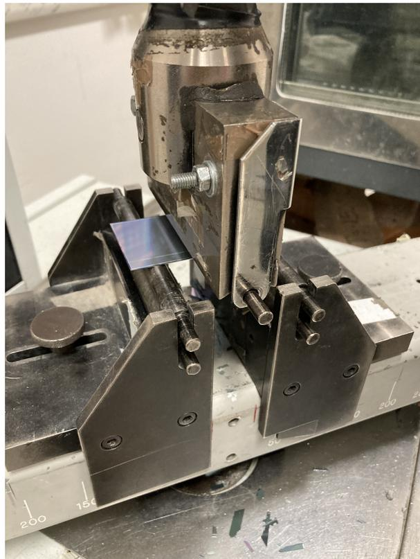
Figure 6. Three-point bending test setup.
