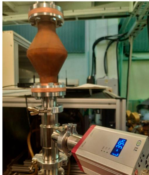
**Figure 4.** Vacuum testing of a test piece with an internal copper coating thickness of about 200  $\mu\text{m}$  and an internal volume of about 1 L.
