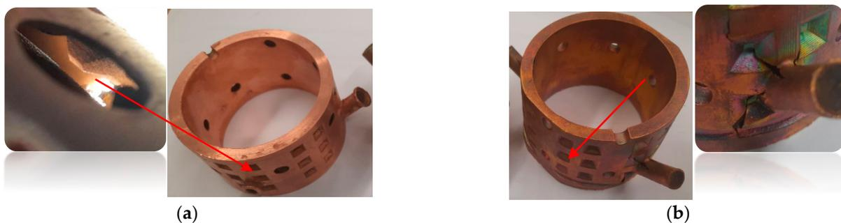
**Figure 8.** Manufactured sectors of the collector: (a) considering the difference in TEC and (b) without.
