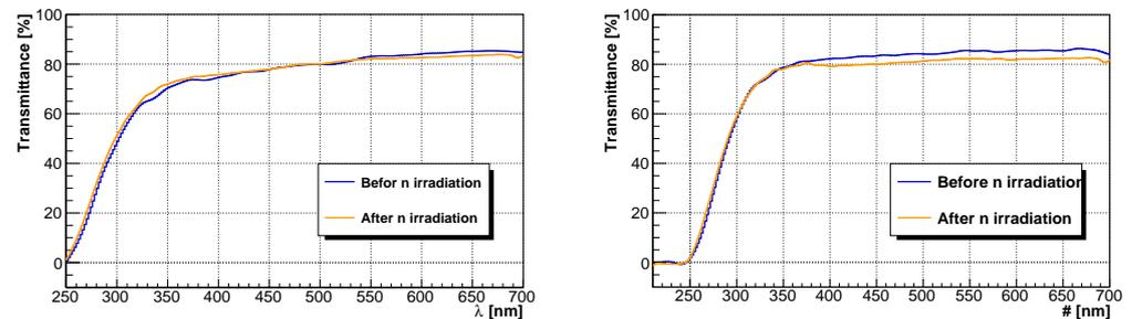
**Figure 6.** Transmission spectra obtained after the irradiation at FNG with 14 MeV neutrons for a total fluence of  $10^{13}$  n/cm<sup>2</sup> (orange line) compared with the results after the 16 hours optical bleaching (blue line) for the naked crystal (left) and for the crystal with Mylar wrapping (right).
