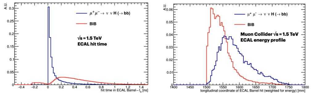
**Figure 1.** The (left) panel shows the time of the ECAL barrel hits with respect to bunch crossing time, for BIB and  $H \rightarrow \bar{b}b$  signal. In the (right) one the energy distribution of ECAL barrel hits as a function of the distance with respect to the beam axis is presented [1].
