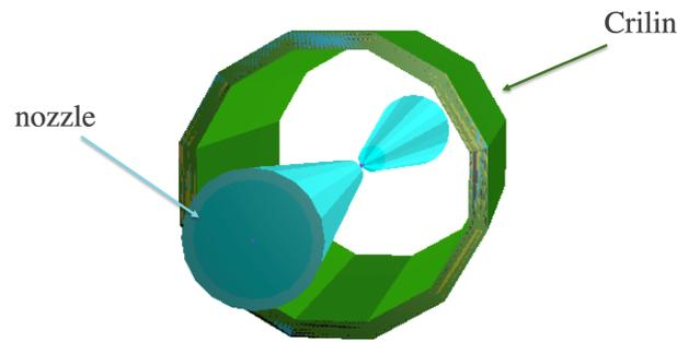
**Figure 2.** Geant4 realisation of Crilin using a dodecahedra geometry together with nozzles.
