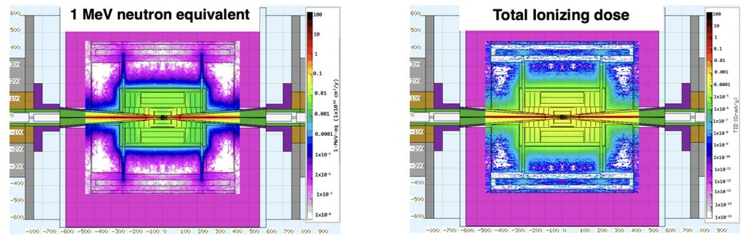
**Figure 4.** (Left): Map of the 1-MeV-neq fluence in the detector region for a Muon Collider operating at  $\sqrt{s} = 1.5$  TeV with the parameters described in [3], shown as a function of the position along the beam axis and the radius. (Right): Map of the TID in the detector region shown as a function of the position along the beam axis and the radius.
