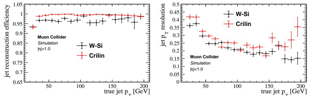
**Figure 3.** (Left): jet reconstruction efficiency as a function of the jet  $p_T$ , obtained by using the Crilin ECAL barrel and the W-Si ECAL barrel. (Right): jet  $p_T$  resolution as a function of the jet  $p_T$ , obtained by using the Crilin ECAL barrel and the W-Si ECAL barrel.
