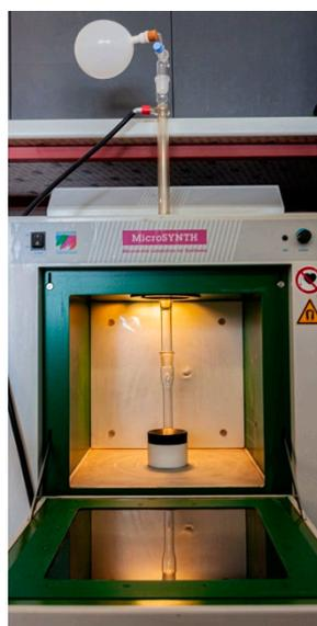
**Figure 3.** Experimental apparatus for 2-aryl-2,3-dihydroquinolin-4(1H)-ones microwave-assisted synthesis.
