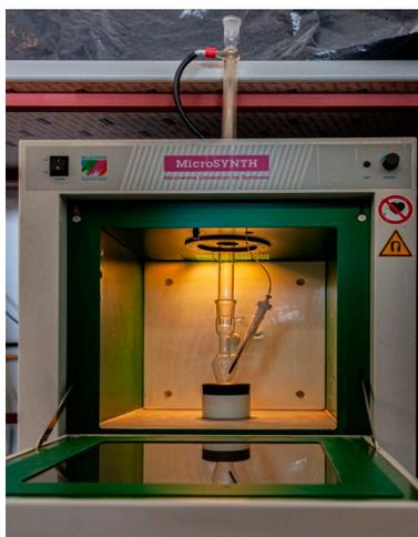
**Figure 1.** Experimental apparatus for microwave-assisted synthesis of chalcone derivatives.
