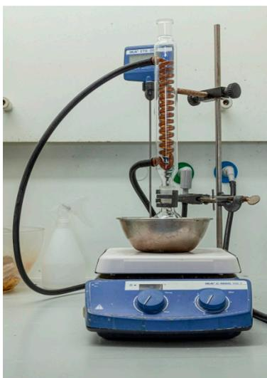
**Figure 2.** Experimental apparatus for the synthesis of flavanones.
