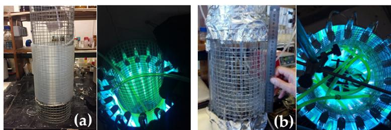
**Figure 1.** Previously reported home-made continuous-flow reactors. (a) FEP4 reactor [(2296 cm (*l*) × 0.4 cm (*d*)] around metal grid (left), and top-view under irradiation (right). (b) Parallel quartz tube reactor (PQT4), [24 tubes in vertical orientation and parallel to each other: 22.5 cm (*l*) × 0.4 cm (*d*)] (left) and top-view under irradiation (right) [7].
