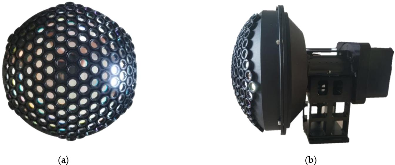
**Figure 6.** (a) The front-view multispectral array and (b) the side view of the prototype BM3C system.
