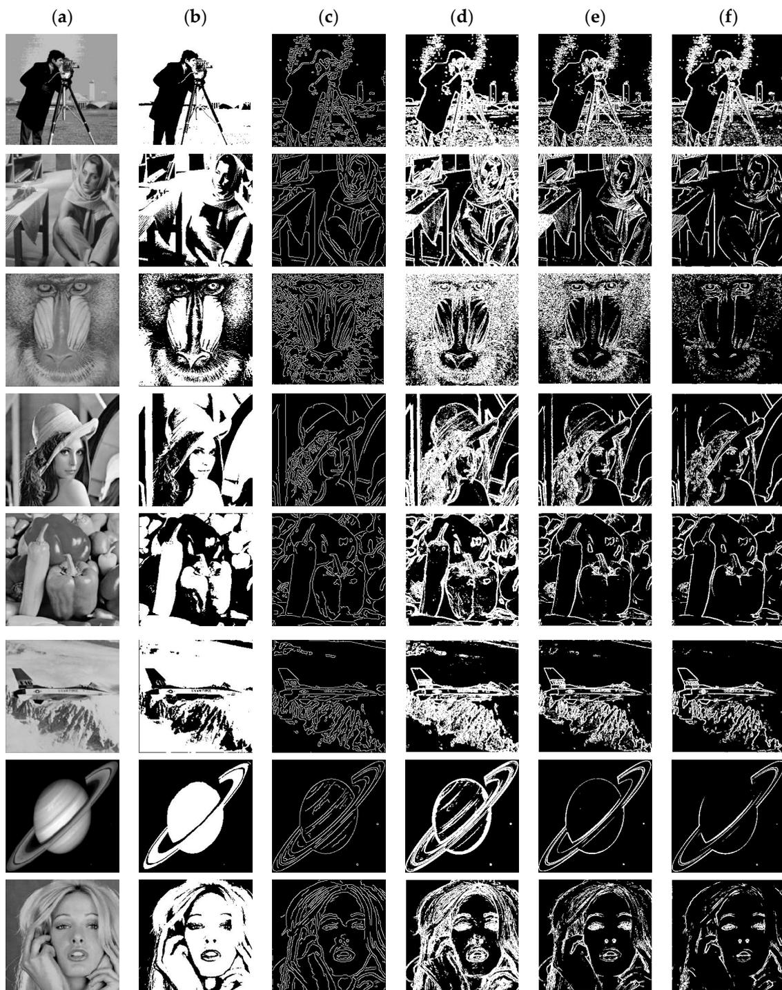
**Figure 2.** (a) Represents the original image and (b) the segmented image with TRDE, (c) the Canny image segmentation method, (d) the Sobel image segmentation method, (e) the Robert image segmentation method, and (f) the Prewitt image segmentation method.
