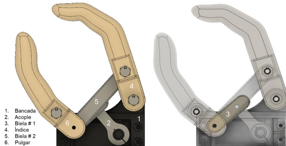
**Figure 8.** Resulting links.
