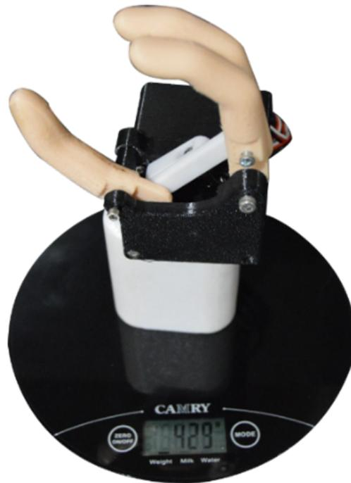
Figure 32. Prototype weight.
