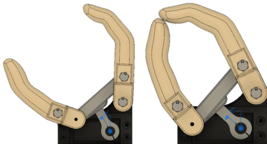
**Figure 9.** Maximum extension (left) and flexion (right).
