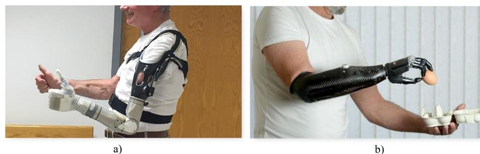
Figure 2. Types of prostheses: (a) Active mechanical prosthesis [16] (b) Electronic active prosthesis [17].
