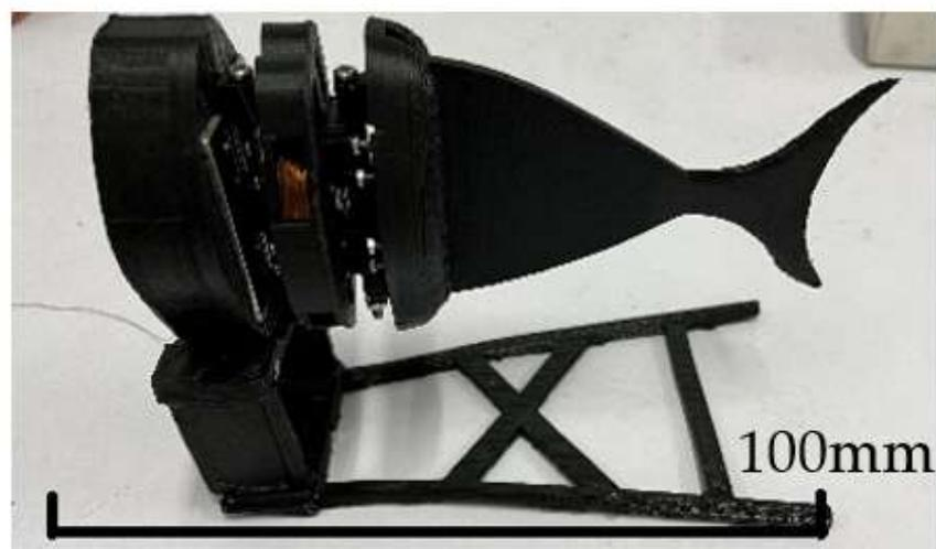
**Figure 7.** Symmetrical bilateral magnetic induction-driven fishtail.
