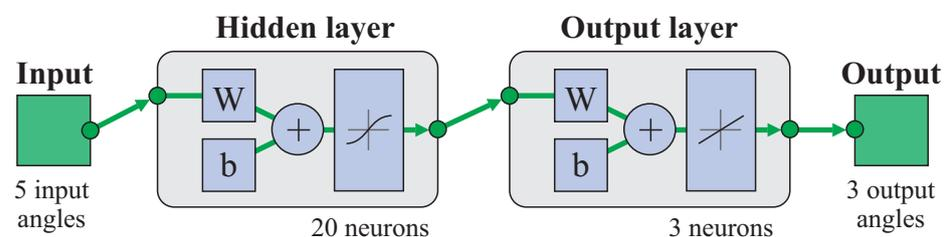
**Figure 4.** FFNN model used (example with 20 neurons in hidden layer, 5 input elbow and shoulder angles and 3 output wrist angles).
