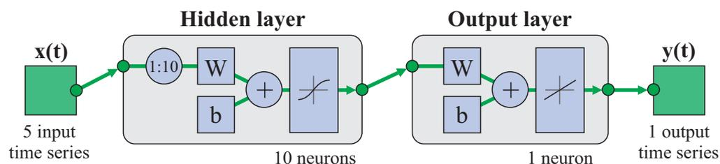
**Figure 5.** Model of TDNN used (example with 10 neurons in hidden layer, 1 time series for one output angle at the wrist, and 5 time series for input angles at the elbow and shoulder). In this case, the network used the previous 10 data points from the time series (1:10).
