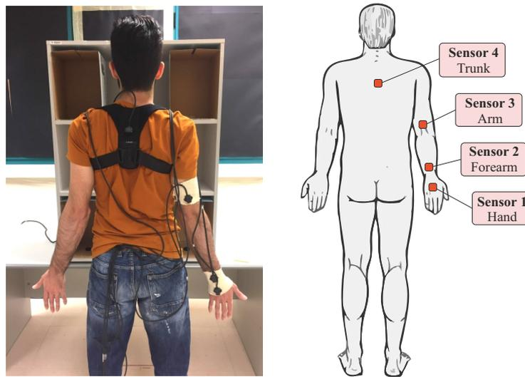
Figure 1. Placement of sensors on the subject.
