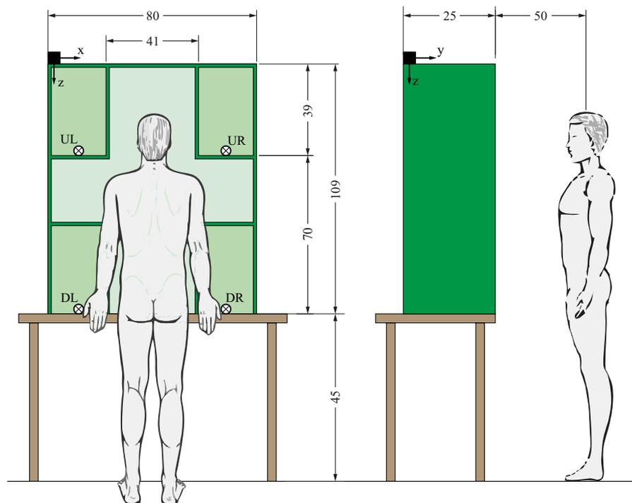
Figure 2. Arrangement of subject and objects during experiments (dimensions in cm).
