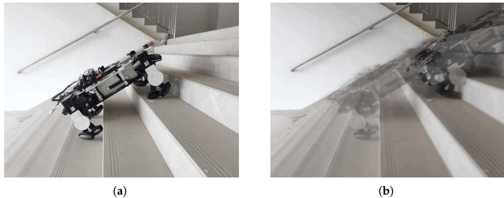
**Figure 15.** LZ-1 uses crawl motion mode to climb stairs.
