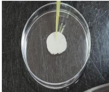
**Figure 3.** Direct contact test on a disk-shaped orthodontic composite sample.
