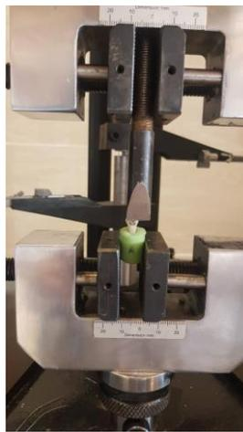
**Figure 2.** Positioning of a sample in the universal testing machine.
