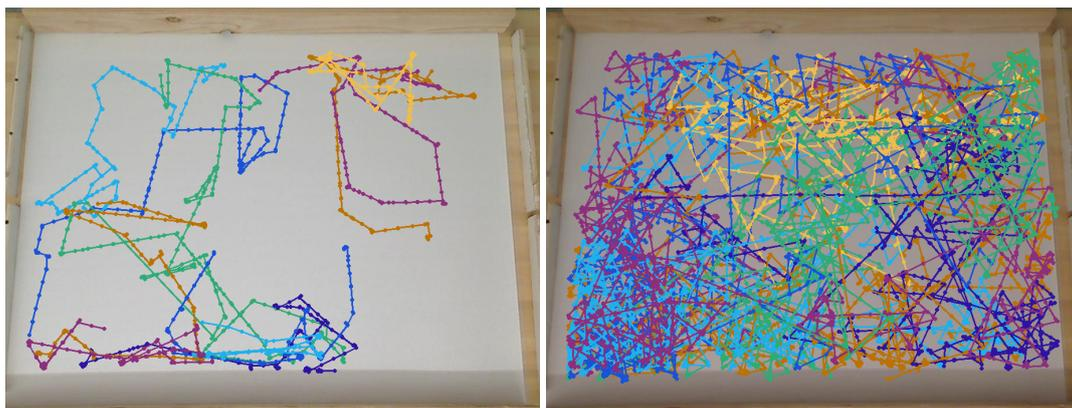
**Figure 21.** Summary of experimental runs on white poster for all 12 initial positions with (left) basic chemotaxis controller and (right) RapidCell controller. Each run is shown in a different color.
