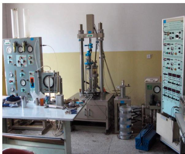
Figure 1. Triaxial equipment for measuring soil properties.
