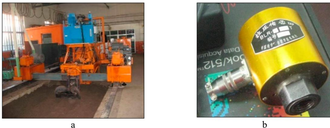
**Figure 5.** Indoor experiment equipment. (a) Indoor experiment electronic carriage; (b) 5 kN force sensor.
