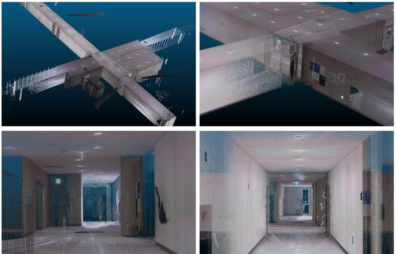
**Figure 12.** Detailed view of the registered point cloud using the proposed methodology.
