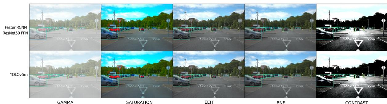
**Figure 4.** Sample detection results from YOLOv5m and Faster RCNN ResNet50 FPN across a subset of ISP configurations. Extreme ISP block configurations were chosen to depict the impact of these blocks on the image. Within the images, the green bounding boxes are ground truth, the blue boxes are detected vehicles, the orange boxes are detected people, and the pink boxes are detected bicycles.
