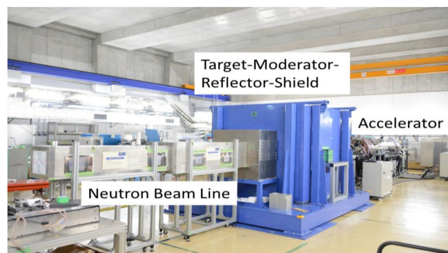
Figure 8. Accelerator, target-moderator-reflector system with shield, and neutron beam line.
