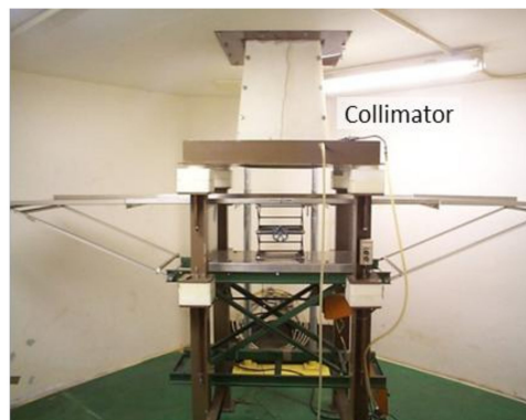
Figure 18. Irradiation area and sample stand.
