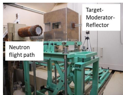
Figure 15. Target-moderator-reflector and neutron flight path.
