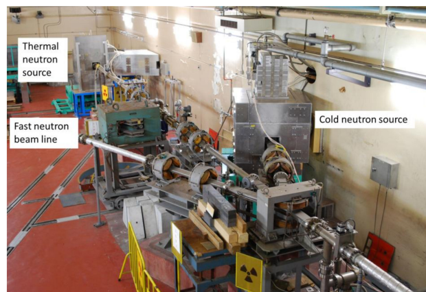
Figure 2. Electron accelerator beam lines at Hokkaido University neutron source. The center beam line is used for thermal neutron experiments, the right for cold neutron ones, and the left for fast neutron ones.
