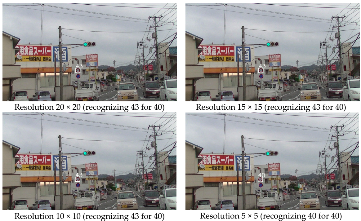
Figure 18. Example of recognition results for 40 km speed-limit sign.
