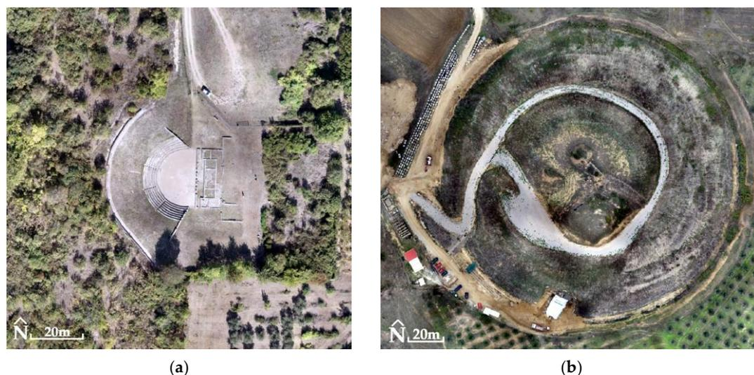
**Figure 15.** (a) The Ancient Theater of Mieza ( $40^{\circ}38'38.6''$  N  $22^{\circ}07'21.3''$  E): orthophotomosaic (true color) without the use of GCPs in the processing of RGB images; (b) the Kasta Mound ( $40^{\circ}50'21.5''$  N  $23^{\circ}51'44.9''$  E): orthophotomosaic (true color) without the use of GCPs in the processing of RGB images.
