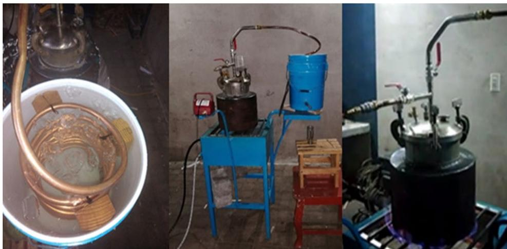
**Figure 2.** Equipment and reactor for pyrolysis.
